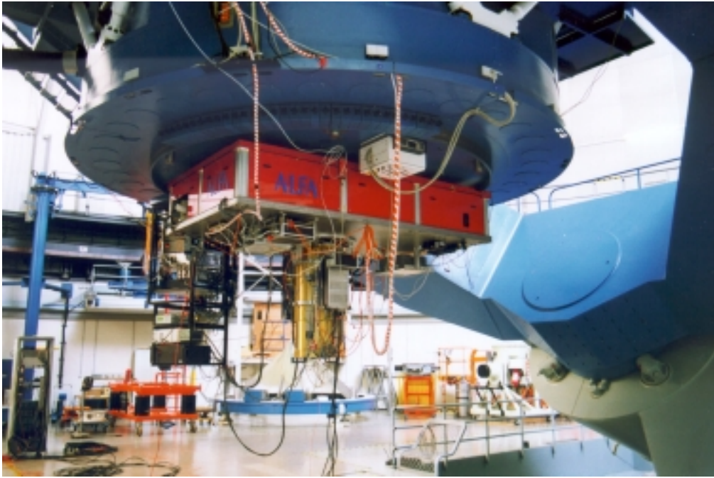
Figure 2. ALFA (rectangular box) and the near-infrared camera OMEGA-Cass (below ALFA) mounted at the Cassegrain flange of the 3.5 m telescope.
