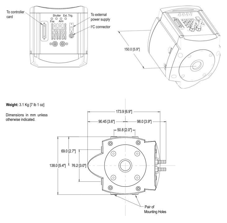
**Note:** The clearance from the C-mount face plate to the shutter is 6mm. Please ensure that when fitting a lens, to a system with a built in shutter, that it does not extend into the housing by more than 5mm.
