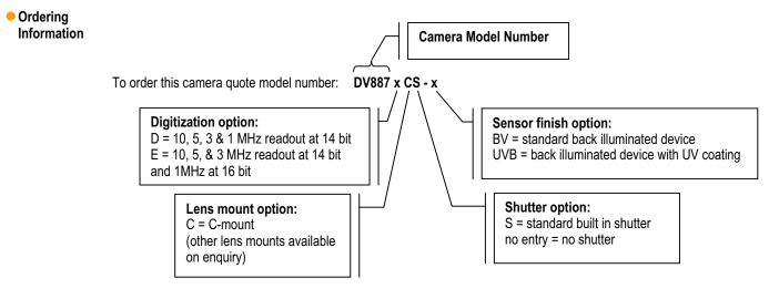
e.g. DV887DCS–UVB a back illuminated iXon DV887 camera with 14-bit digitization at 10, 5, 3 and 1MHz readout speeds, EMCCD and conventional output amplifiers, standard shutter and UV-enhanced coating.
