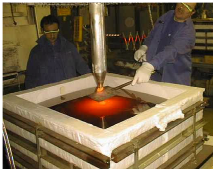
Fig. 3: N-BK7 block glass (left) Fig. 4: Casting of radiation shielding windows (middle) Fig. 5: Large N-BK 7 boules (right)
