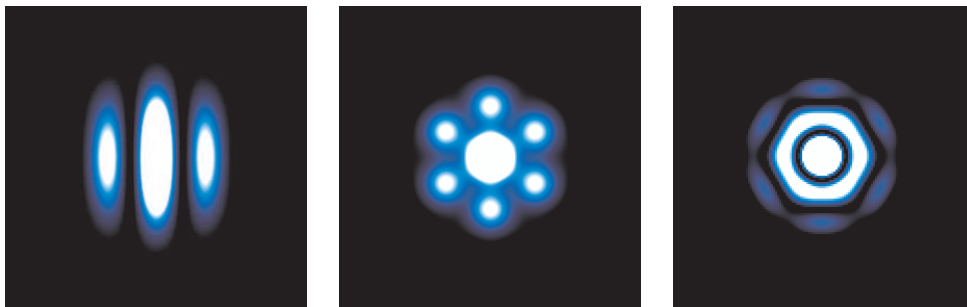
Figure 2. Calculated PSFs of the corresponding aperture geometries of Fig. 1. Left to right: A single exposure of the LBT; a numerically combined triple-exposure of the LBT; a single exposure of the OWL telescope using a segmented M5 mirror. The segmentation of OWL’s primary mirror has been neglected for the calculation since its segmentation is more than a magnitude finer than the one of the M5 mirror.
