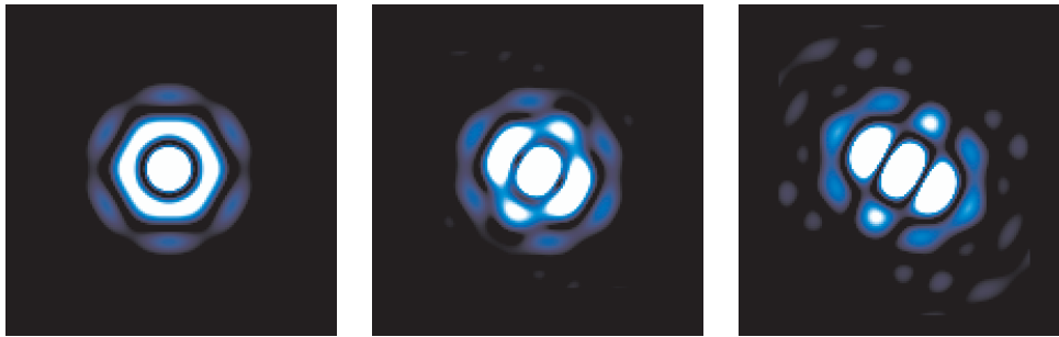
Figure 3. Calculated PSFs of the OWL telescope using a modularised M5 with an increasing number of absent segments. Left to right: All 6 segments in diffraction limited closed loop operation; 5 operative segments; 4 operative segments with the 2 absent ones located on opposite sides of the aperture.
