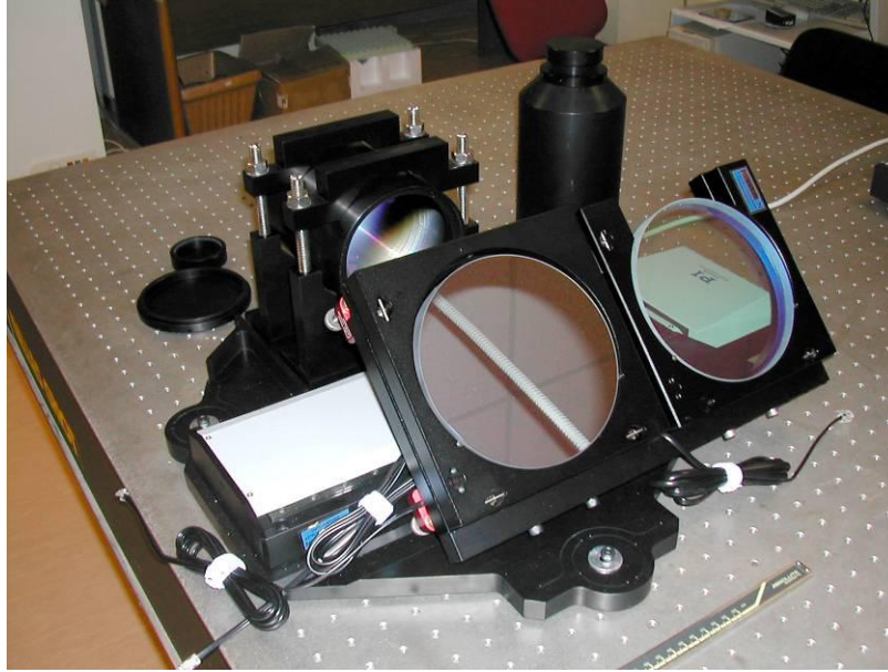
Figure 10: The Patrol Camera opto-mechanics mounted in Rome Observatory laboratory
