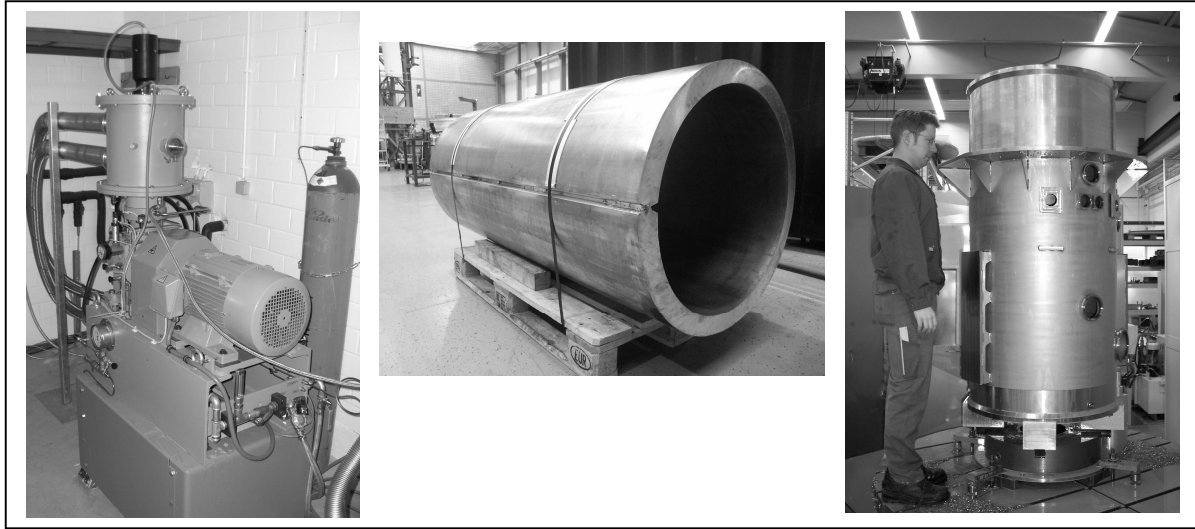
Figure 11 left: Stirling cooler at the MPIA; middle: Aluminum cylinder for the heat exchanger; right: vacuum can on the machine
