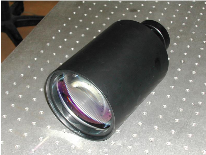
Figure 8. Mechanical mounting of the camera optics.
