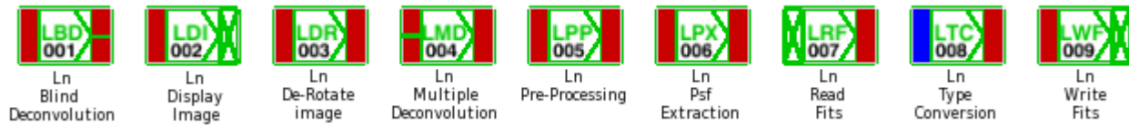
Figure 1. List of modules composing AIRY-LN. Each of them admits from zero to two inputs or outputs, colored within the CAOS Application Builder as seen here (red if for the ad-hoc-defined “LN data” type and blue for the already existing “image” type used in AIRY_4.0).
