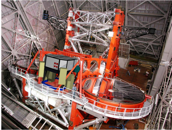
Figure 1: The LBT nearing completion in January 2006. LINC-NIRVANA is the large, light gray box at the shared focal station closest to the viewer (installed courtesy of Photoshop). Note the human figure for scale.
