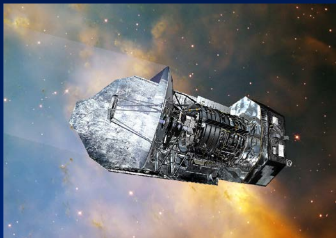
The Herschel Satellite by ESA with its 3.5-m mirror
