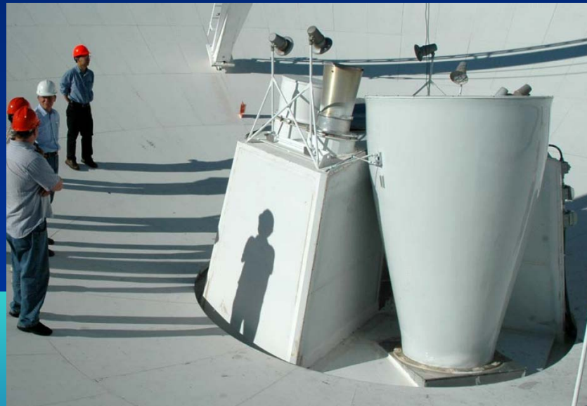
Different feed horns in the main dish of a VLA antenna
