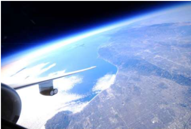
Figure 1 - Two round, large-area cosmic dust collectors deployed beneath the wing of a NASA ER-2 aircraft in flight.
