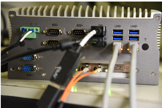
Figure 30: Example of a OPTPCI-e board horizontally installed in a PicoSys 2614.
