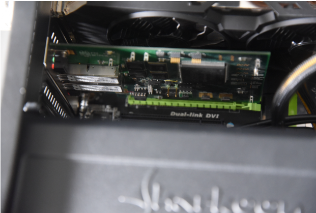
Figure 33: Example of a OPTPCI-e board vertically installed in a Sharkoon A10-7850K.
