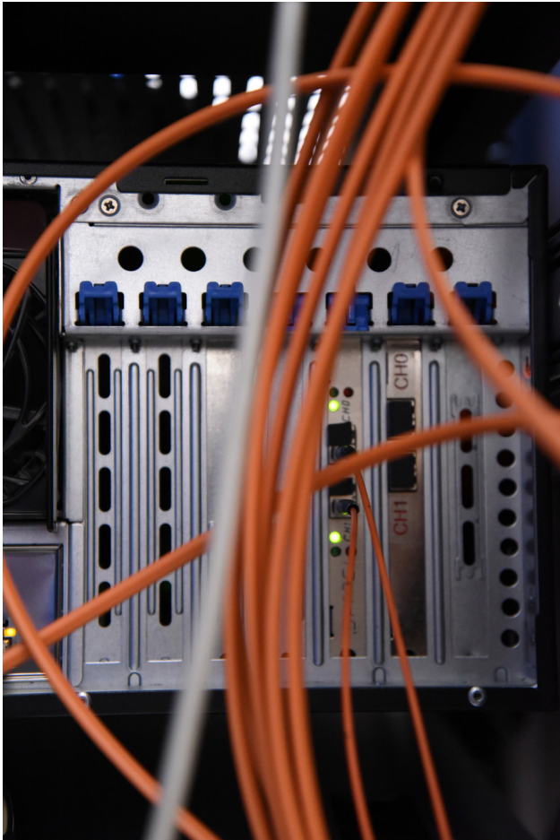
Figure 29: Example of two OPTPCI-X boards vertically installed in a Transtec Workstation (2 Opteron-4C, 2382).
