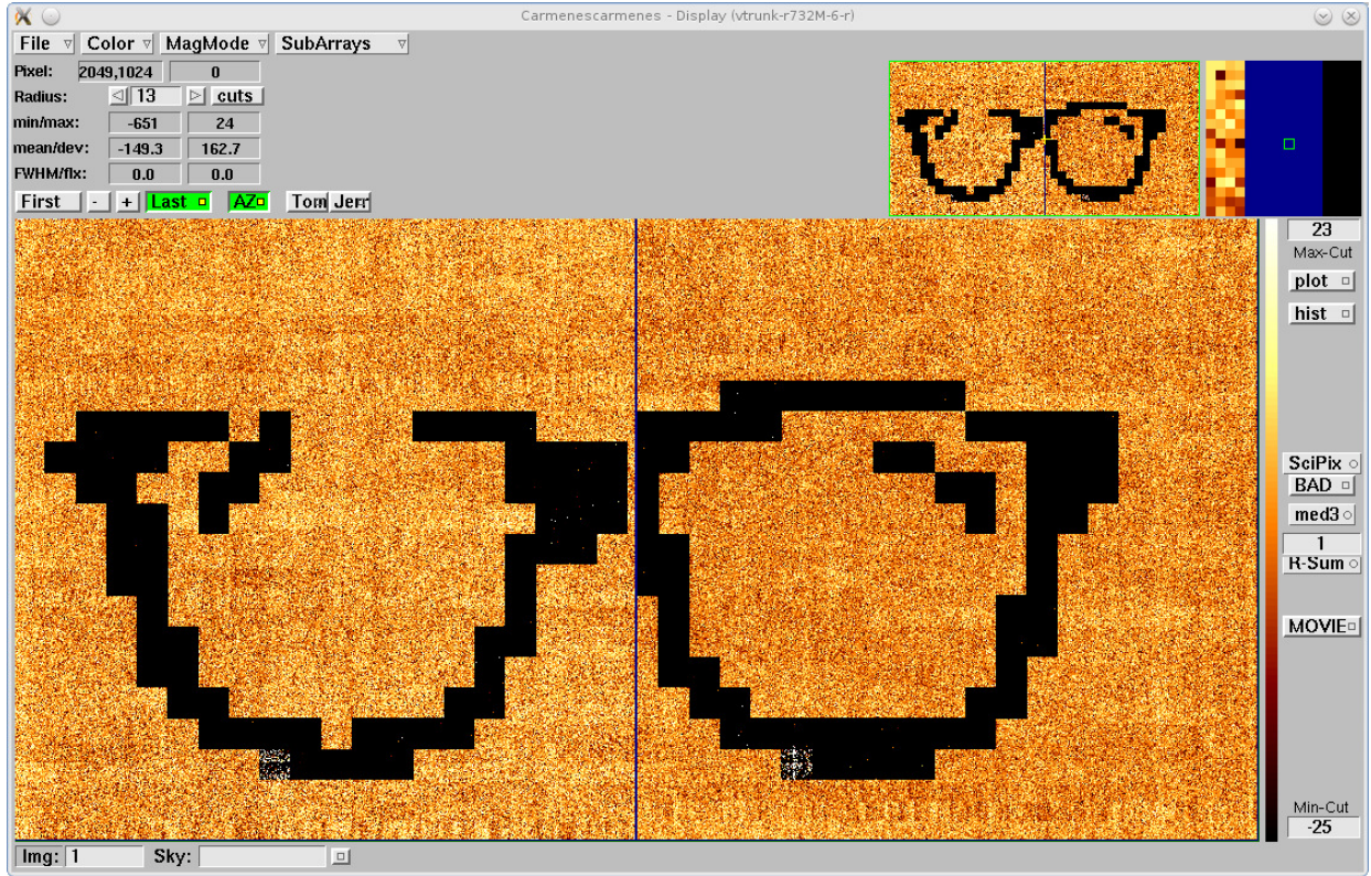
Figure 20: The CARMENES image generated by the linear fit through 4 frames (see Section 5.6.2.3) associated with Figure 19.
