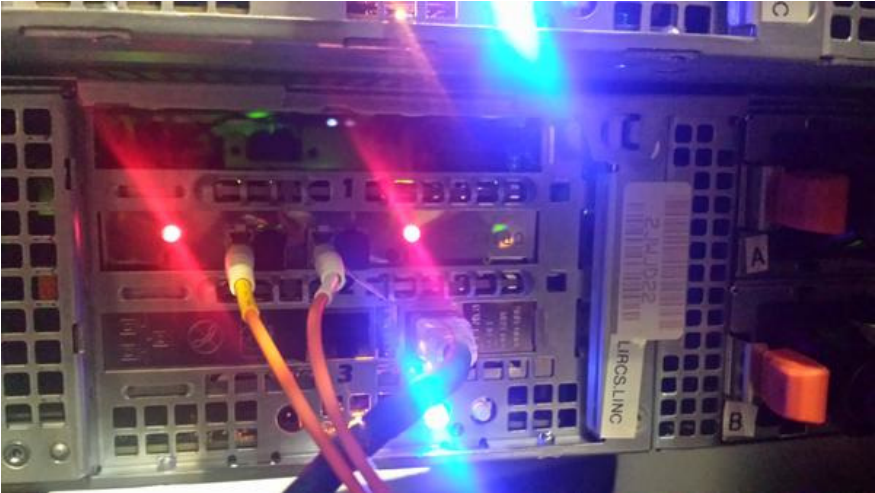
Figure 32: Example of a OPTPCI-e board horizontally installed in a Dell PowerEdge R515. The two fibers are likely at the wrong places in this photo, which means they are plugged in the “send” ports of the two OPTPCI-e ports, but should be plugged into the “receive” ports to get a working system.
