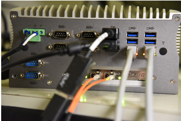
Figure 35: Example of a OPTPCI-e board horizontally installed in a PicoSys 2614.
