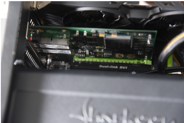
Figure 38: Example of a OPTPCI-e board vertically installed in a Sharkoon A10-7850K.
