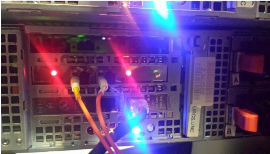
Figure 37: Example of a OPTPCI-e board horizontally installed in a Dell PowerEdge R515. The two fibers are likely at the wrong places in this photo, which means they are plugged in the “send” ports of the two OPTPCI-e ports, but should be plugged into the “receive” ports to get a working system.
