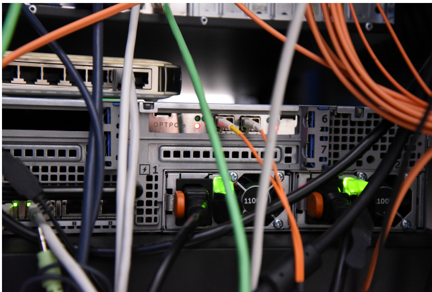
Figure 36: Example of a OPTPCI-e #015 board horizontally installed in a Dell PowerEdge R720.
