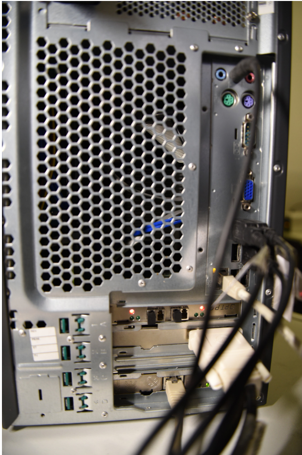
Figure 39: Example of a OPTPCI-e board horizontally installed in a Fujitsu Siemens Esprimo P7935. The board was de-installed in Oct 2020.
