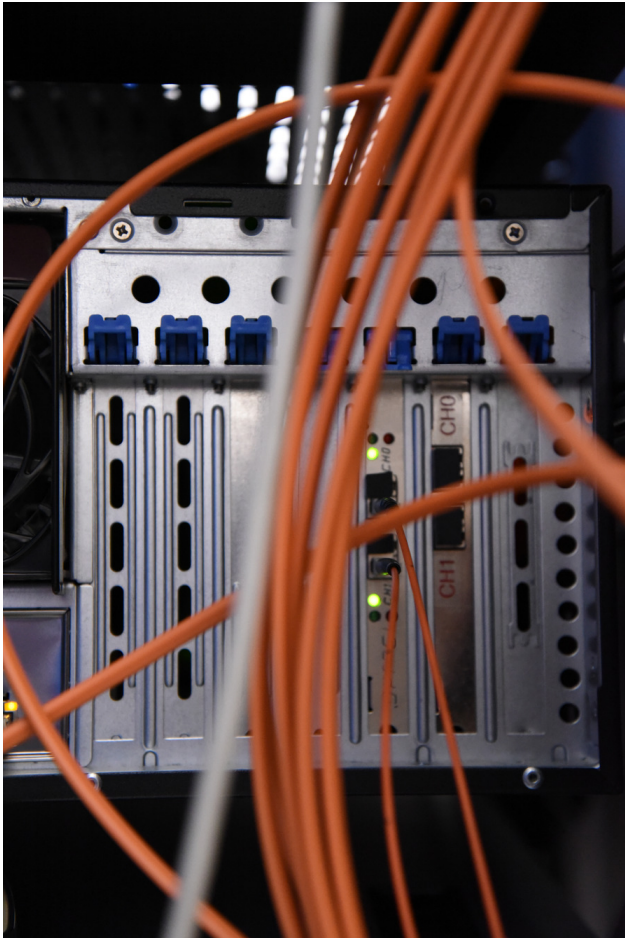
Figure 34: Example of two OPTPCI-X boards vertically installed in a Transtec Workstation (2 Opteron-4C, 2382).
