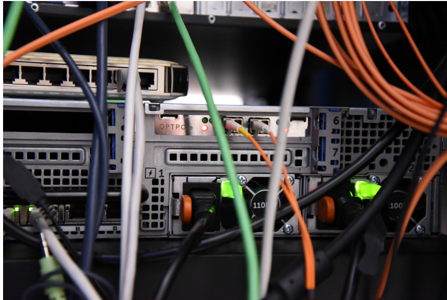
Figure 31: Example of a OPTPCI-e #015 board horizontally installed in a Dell PowerEdge R720.
