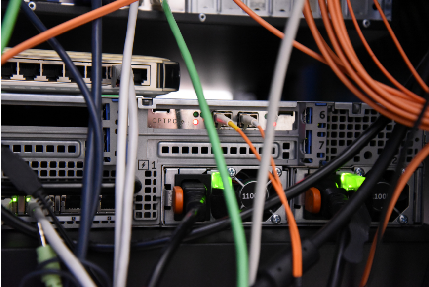
Figure 38: Example of a OPTPCI-e #015 board horizontally installed in a Dell PowerEdge R720.
