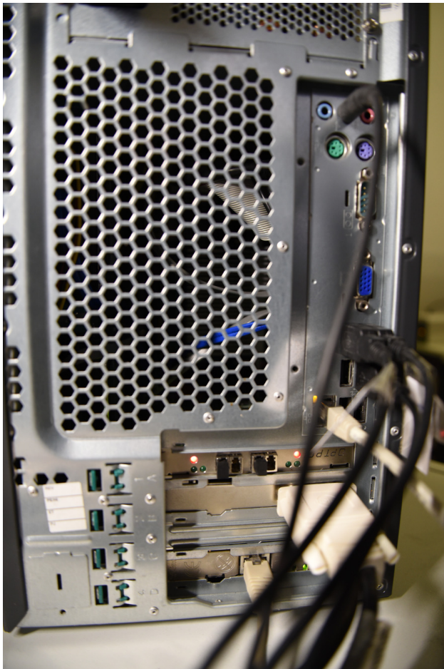
Figure 41: Example of a OPTPCI-e board horizontally installed in a Fujitsu Siemens Esprimo P7935. The board was de-installed in Oct 2020.
