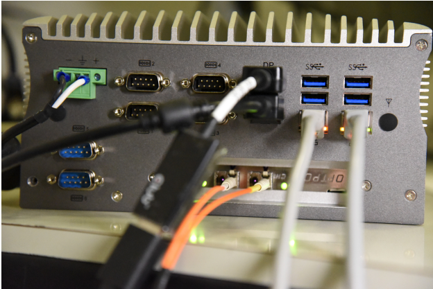
Figure 37: Example of a OPTPCI-e board horizontally installed in a PicoSys 2614.
